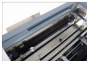
Jobs can be cross-perforated by swapping out the creasing unit with the cross-perforating unit.
