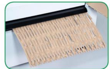
Produces flexible perforated cardboard netting, at speeds of up to 34 fpm
