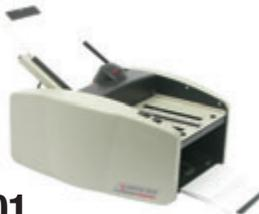
The 1601 automatic paper folder is great for mailrooms and offices and is simple to operate. It can quickly fold a variety of documents and can create up to 5 of the most common folds such as the letter, half, z-fold, double parallel and french. It operates at a speed of 9,000 sheets per hour. It holds up to 150 sheets in the paper tray at once. Improvements in the fold plate settings allow for precise folds and easy adjustments.
