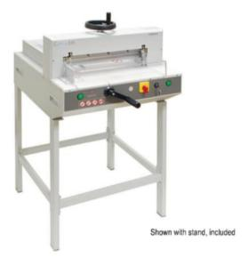
The Formax Cut-True 22S Electric Paper Cutter offers precision cutting for paper stacks up to 16.9" wide. This semi-automatic cutter requires very little effort, thanks to its electronically-controlled two-button operation. Simply load a stack of paper, up to 1.75" high, secure with the geared clamp, and press the buttons to engage the hardened-steel Guillotine blade.
